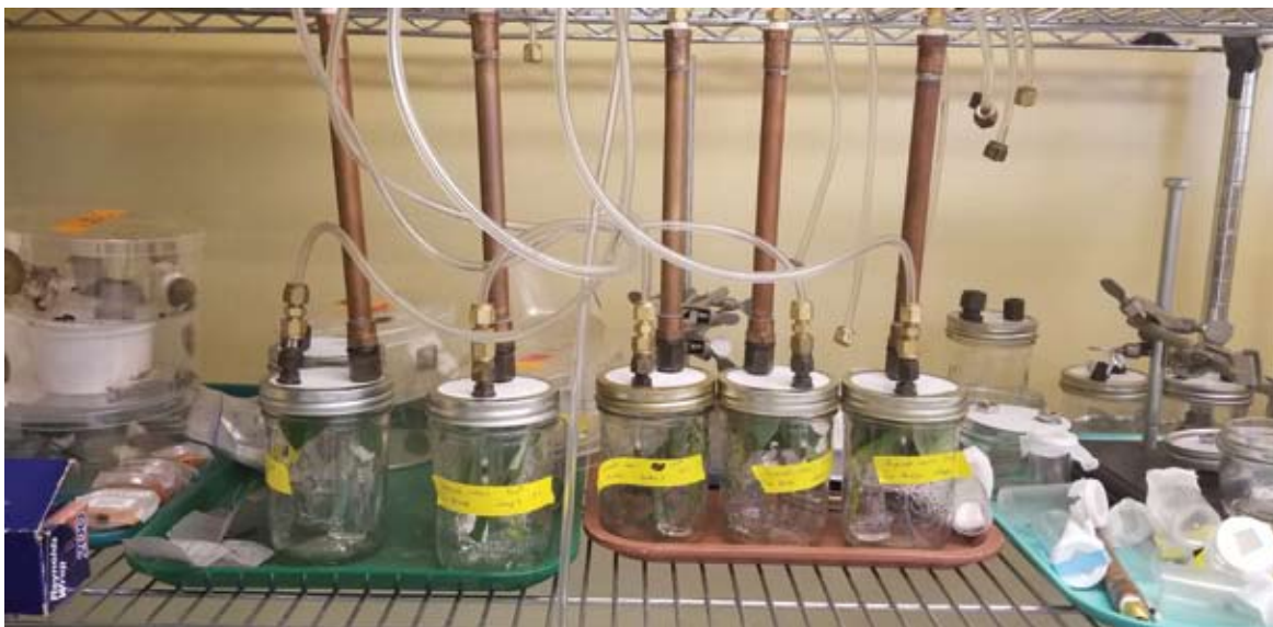
Aeration chambers in quarantine set up to capture H. lauri aggregation pheromones.
