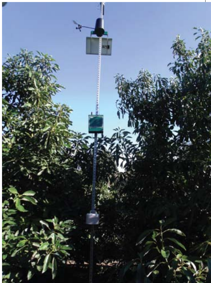
A base station determines ET by tracking variables like temperature, humidity, wind speed, wind direction and rain.
