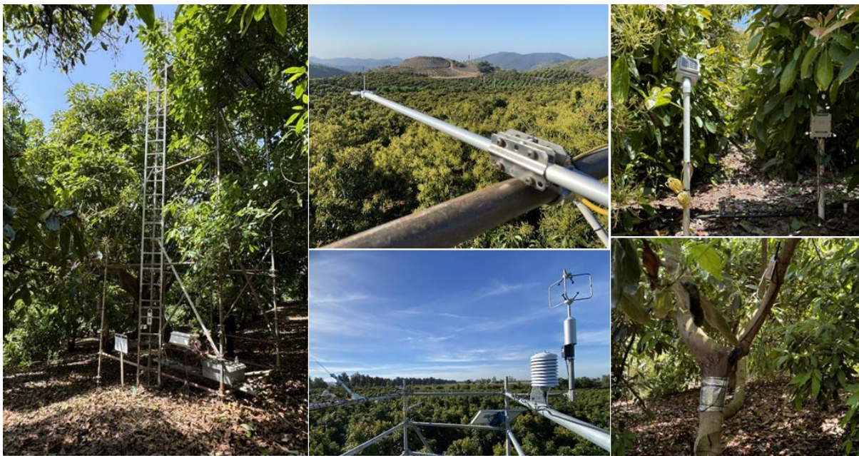
Fig. 1. A demonstration of flux tower monitoring station and some of the instrumentation set up.
