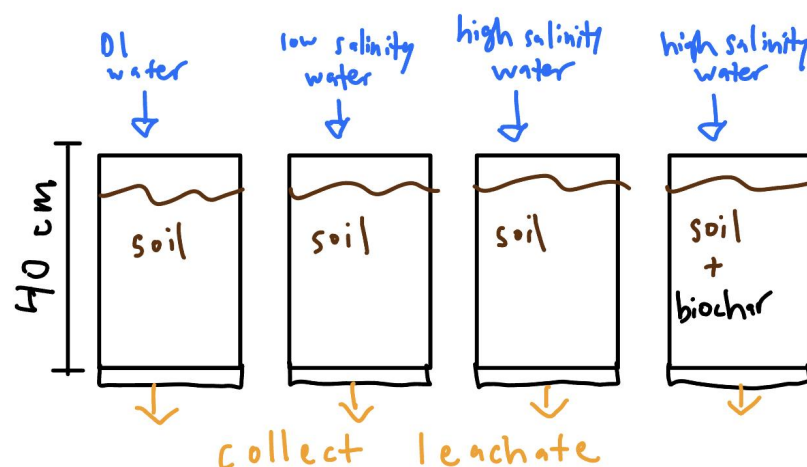
Figure 2: Soil column laboratory experiment set up with soils collected from six different sites
