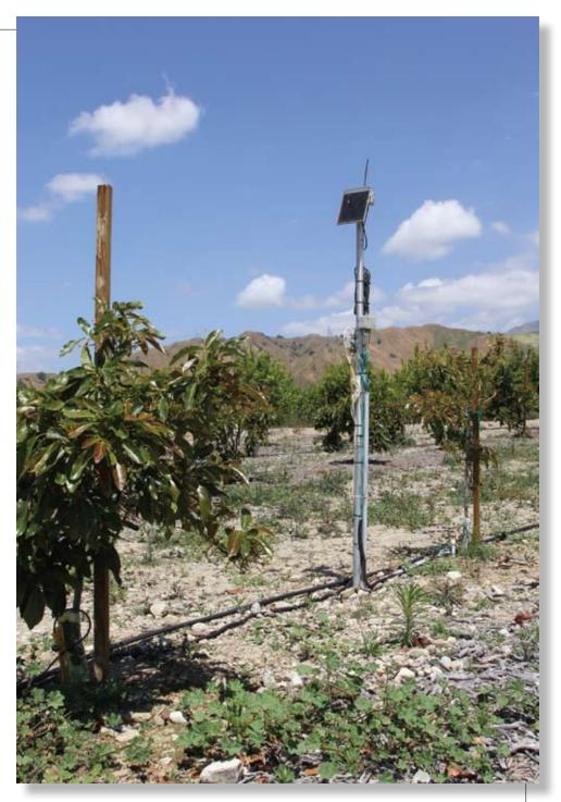
An in-field data logger and radio station used to record and transmit soil moisture sensor data back to the base station.
