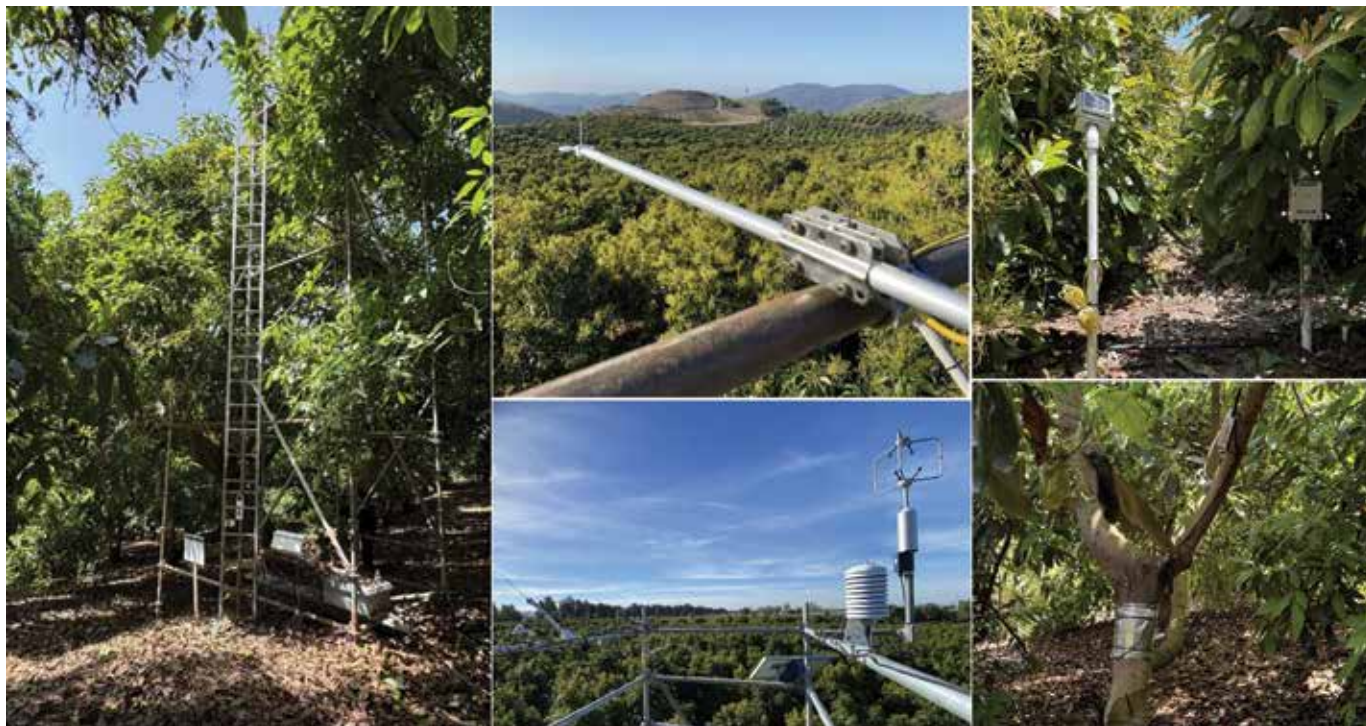
Fig. 1. A demonstration of one flux tower monitoring station and some of the instrumentation setup.
